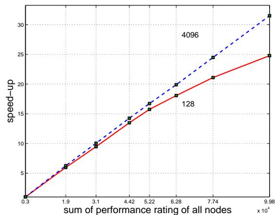
Figure 2. Comparison of speed-ups for two sets of experiments involving 128 and 4096 samples.
