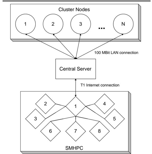
**Figure 1. Diagram of how the nodes of the cluster are connected to the central server which is connected to the shared-memory high performance computer (SMHPC).**
