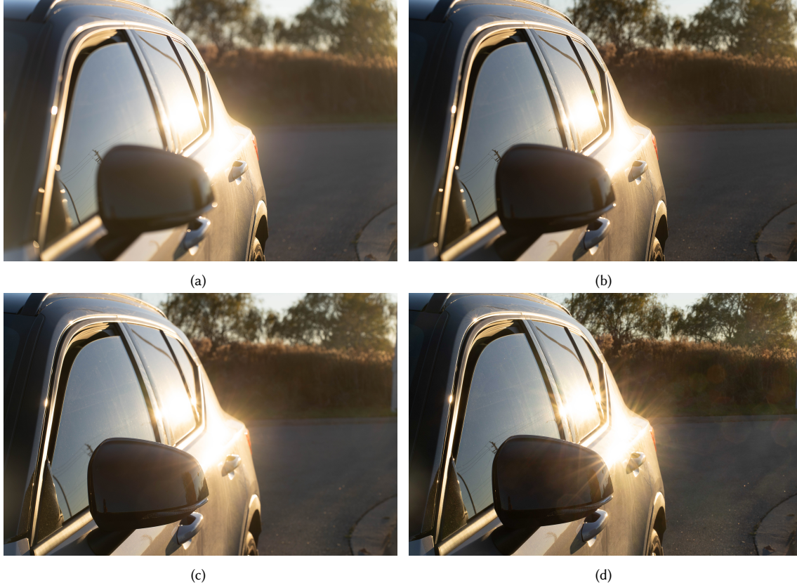
Fig. S3. A sequence of photos taken by a camera during daytime to show the camera version of glare patterns. The patterns could be observed around the specular reflection spots. The photos presented in Figs. (a), (b), (c), and (d) correspond to aperture sizes f/\# equal to f/2.8 , f/5.6 , f/11 , and f/22 , respectively.
