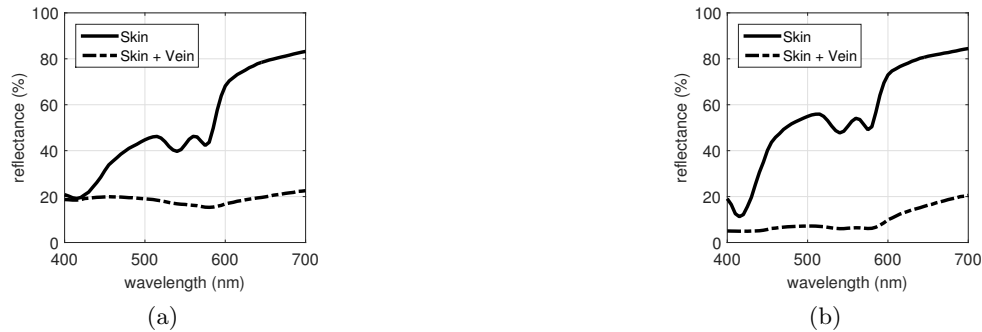
Figure 5. Modeled reflectance curves obtained for the baseline skin specimen with and without a subcutaneous vein. (a) With Rayleigh scattering. (b) Without Rayleigh scattering.
